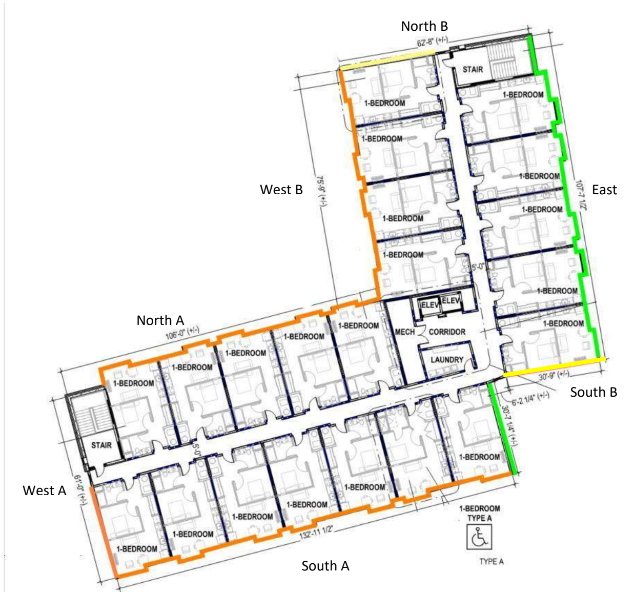
Figure 5: Building Facade DNL levels with Orange for DNL >70 to 75, Yellow for DNL >65 to 70, both considered “Normally Unacceptable”, and Green for DNL 65 or less, considered “Acceptable”.
